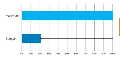
Sandvik OH68 shows up to 80 % less wear than the maximum allowed in industry-standard hydraulic pump test.
